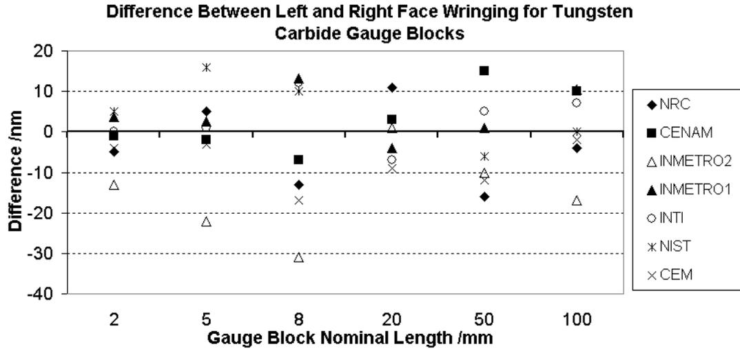
Figure 4: Plot of differences between left and right wringing compared to average central length for each participant, for tungsten carbide gauge blocks.
