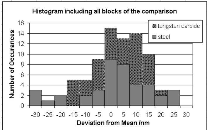
Figure 5: Histogram combining all gauge blocks of the comparison. Number of occurrences of difference value from the simple arithmetic mean.
