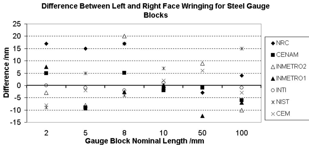
Figure 3: Plot of differences between left and right wringing compared to average central length for steel gauge blocks.
