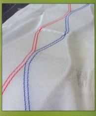
Components made from warp-knitted spacer textiles by Karl Mayer; for the purpose of demonstrating the technology, coloured pile yarns are used to show the guiding of both pile guide bars when working the contours.
