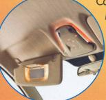
Nonwovens based on bast and cellulosic fibres as substrates for composites, such as Johnson Controls AE's glass-free headliner (Ecobond), have come a long way in the past twenty years.
