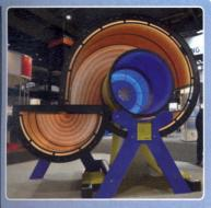
Fleissner's Streamliner is a through-air dryer with a highly uniform, spiralling airflow passing through the fabric. This is one of a number of ways nonwovens machinery builders are addressing the issue of reducing the use of energy for their customers, according to
