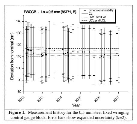
This fixed wringing control gauge block was manufactured several years before this control measurement was started hence the data show the 0,5 mm control gauge block is very stable, as it was expected.
