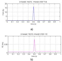
Figure 6. Phase step results referred to: a) Response time. b) Delay.
