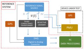
Figure 1. Scheme of INTI PMU calibration system.
